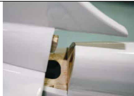
Use those 3 bigger screws with nuts for rudder control horns
