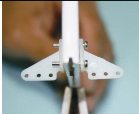
Install pull-pull rudder control horns
