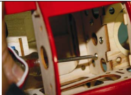
Install mount box to the fuselage.
