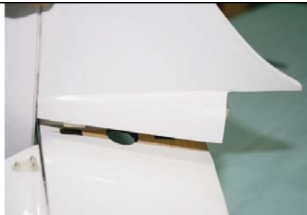
Install vertical stabilizer
