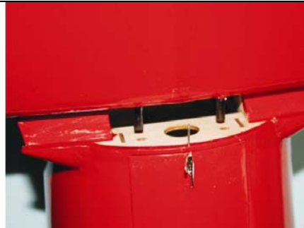
Install wing to the fuselage
