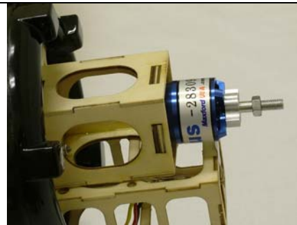
Motor mount was designed with a little bit down thrust.
