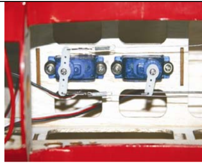
Use the push rod for elevator, rudder is pull-pull.
