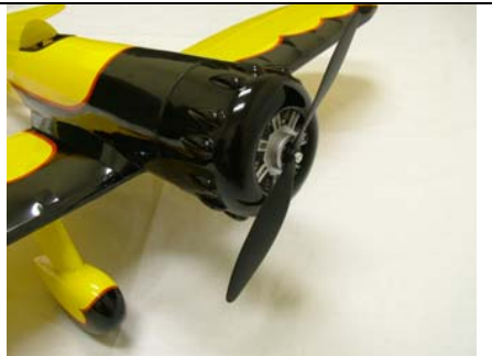
Install fiberglass cowl.
